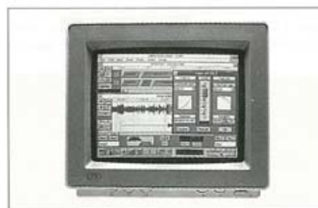
A page from Sadie disk editor system from Studio Audio and Video Ltd.
